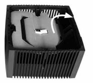
Remove the disc stack(s) from the lower housing and set them aside. Remove the protective cardboard from the upper and lower housings. Check the lower housing and the disc stack(s) for any cracks or damages. If everything is fine, put the disc stack(s) back in the lower housing.
