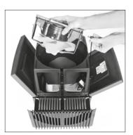
Lift the motor out of the housing, remove the power cable, and set it aside for a moment.
