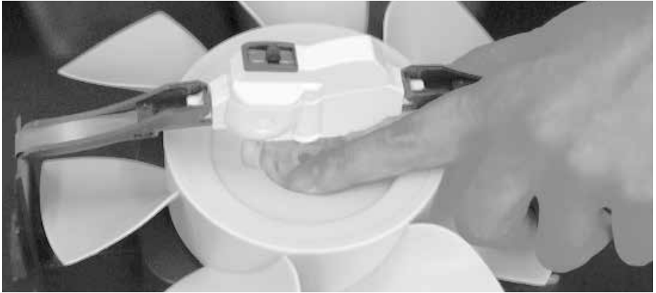
Fig 4. ... Push the coupling down ...
