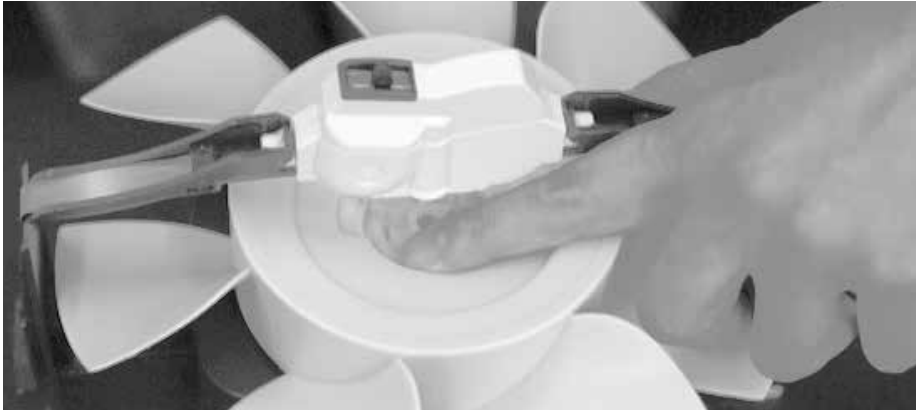
Fig 4. ... Push the coupling down ...
