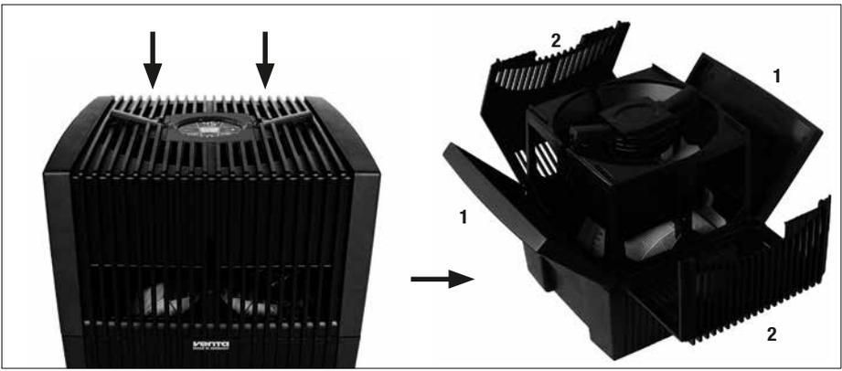
Open the top of your Airwasher by releasing the tabs on the control panel and opening the four panels, starting with the non-vented panels.
